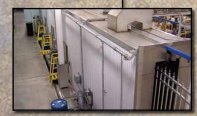
The next four stages consist of a: STEP #3: (CLEAN) City water rinse, STEP #4: (CLEANER) Recycling reverse osmosis water rinse, STEP #5: (CLEANEST) Pure reverse osmosis water rinse. STEP #6: Titanium and zirconium conversion coating with fluoride. STEP #7: (CLEANEST) Pure reverse osmosis water rinse.
